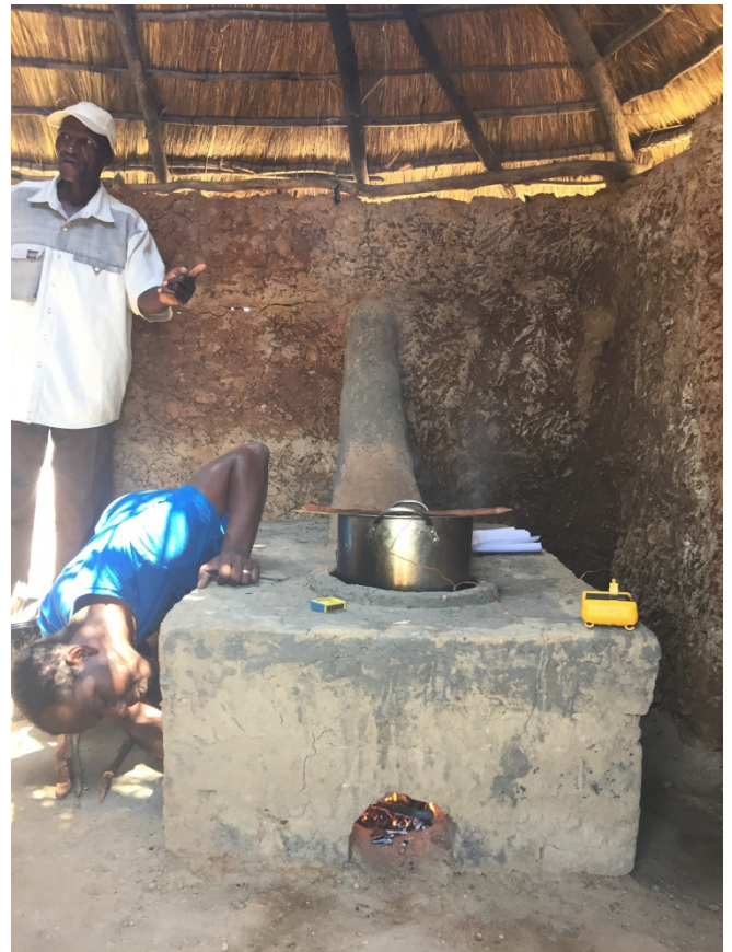
Lecturer from NEI-NUST testing the energy efficiency of the improved stove in Sikondo, Kavango East region.
