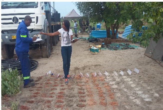
MAWF Hydrologist taking mud samples during drilling
