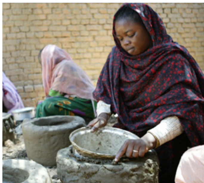
This is a stove being built with clay using old metal tins as moulds.
