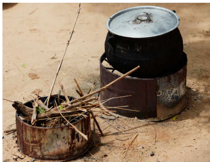
This is a simple metal can stove for people who keep moving from place to place. Take care to use smaller pots so the tin does not tip over and surround the tin with stones to make it more stable.
