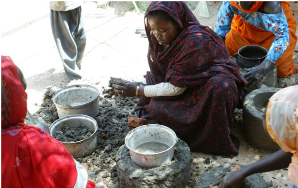
Basic improved stoves can be made with locally available materials at almost no cost: displaced women in Western Darfur, the Sudan, learn how to make fuel-efficient stoves out of mud.
